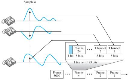
T-1:  $8000 \text{ frames/s} = 8000 \times 193 \text{ bps} = 1.544 \text{ Mbps}$
