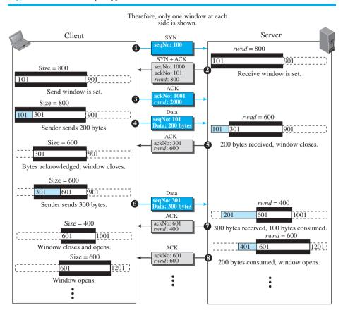
Eight segments are exchanged between the client and server:
