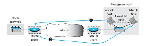
However, when the remote host sends a packet to the mobile host, the packet goes from the remote host to the home agent and then to the mobile host. The packet travels the two sides of a triangle, instead of just one side (see Figure 19.20).
