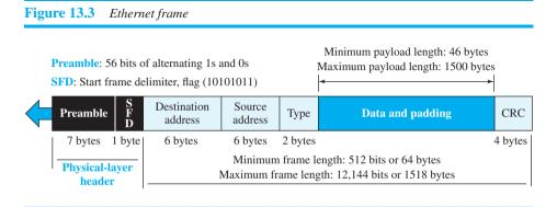
Preamble. This field contains 7 bytes (56 bits) of alternating 0s and 1s that alert the receiving system to the coming frame and enable it to synchronize its clock if it's out of synchronization. The pattern provides only an alert and a timing pulse. The 56-bit
