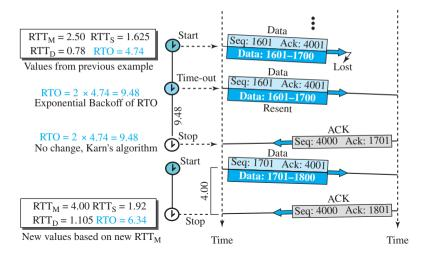
The first segment in the figure is sent, but lost. The RTO timer expires after 4.74 seconds. The segment is retransmitted and the timer is set to 9.48, twice the previous value of RTO. This time an ACK is received before the time-out. We wait until we send a new segment and receive the ACK for it before recalculating the RTO (Karn's algorithm).
