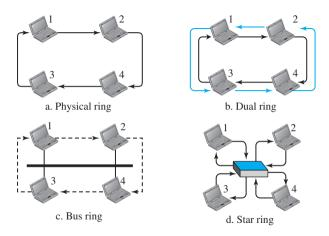
In the physical ring topology, when a station sends the token to its successor, the token cannot be seen by other stations; the successor is the next one in line. This means that the token does not have to have the address of the next successor. The problem with this topology is that if one of the links—the medium between two adjacent stations—fails, the whole system fails.
