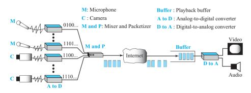
Although it could have only one microphone and one audio player, today's interactive real-time application is normally made up of several microphones and several cameras. The audio and video information (analog signals) are converted to digital data. The digital data created from different sources are normally mixed and packetized. The
