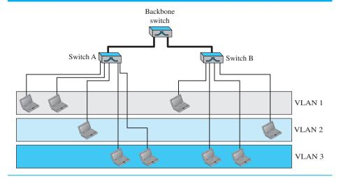
This is a good configuration for a company with two separate buildings. Each building can have its own switched LAN connected by a backbone. People in the first
