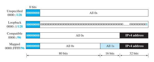
The unspecified address is a subblock containing only one address, which is used during bootstrap when a host does not know its own address and wants to send an inquiry to find it (see DHCP section).
