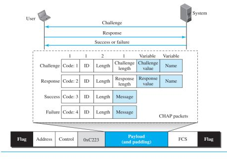
CHAP packets are encapsulated in the PPP frame with the protocol value C223 in hexadecimal. There are four CHAP packets: challenge, response, success, and failure. The first packet is used by the system to send the challenge value. The second is used by the user to return the result of the calculation. The third is used by the system to allow access to the system. The fourth is used by the system to deny access to the system.
