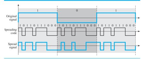
In Figure 6.33, the spreading code is 11 chips having the pattern 10110111000 (in this case). If the original signal rate is N, the rate of the spread signal is 11N. This means that the required bandwidth for the spread signal is 11 times larger than the bandwidth of the original signal. The spread signal can provide privacy if the intruder does not know the code. It can also provide immunity against interference if each station uses a different code.
