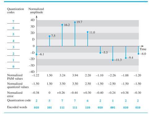
Figure 4.26 Quantization and encoding of a sampled signal
