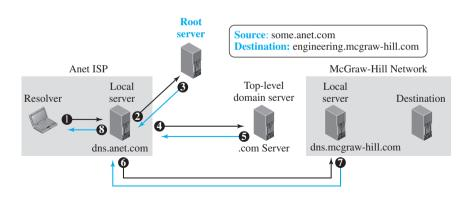
server, and the message shown by event 7 contains the IP address of the destination. When the Anet local DNS server receives the IP address of the destination, it sends it to the resolver (event 8).
