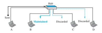
packet from all outgoing ports except the one from which the signal was received. In other words, the frame is broadcast. All stations in the LAN receive the frame, but only station B keeps it. The rest of the stations discard it. Figure 17.2 shows the role of a repeater or a hub in a switched LAN.
