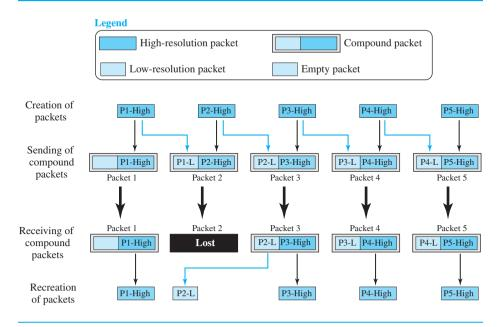
Figure 10.22 Compounding high- and low-resolution packets
