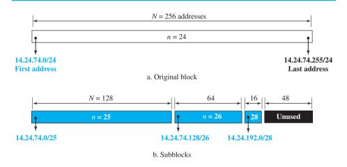
Figure 18.24 Example of address aggregation
