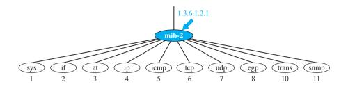
The objects in MIB2 are categorized under several groups: system, interface, address translation, ip, icmp, tcp, udp, egp, transmission, and snmp (note that group 9 is deprecated). These groups are under the mib-2 object in the object identifier tree. Each group has defined variables and/or tables.
