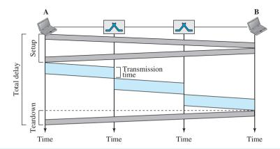
The packet is traveling through two switches (routers). There are three transmission times (3T), three propagation times  $(3\tau)$ , data transfer depicted by the sloping lines, a setup delay (which includes transmission and propagation in two directions),
