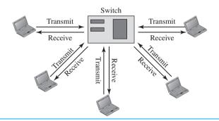
Each station or switch can send and receive independently without worrying about collision. Each link is a point-to-point dedicated path between the station and the switch. There is no longer a need for carrier sensing; there is no longer a need for collision detection. The job of the MAC layer becomes much easier. The carrier sensing and collision detection functionalities of the MAC sublayer can be turned off.
