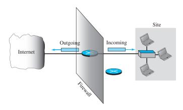
For example, a firewall may filter all incoming packets destined for a specific host or a specific server such as HTTP. A firewall can be used to deny access to a specific host or a specific service in the organization. A firewall is usually classified as a packet-filter firewall or a proxy-based firewall.
