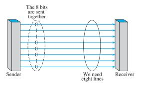
The advantage of parallel transmission is speed. All else being equal, parallel transmission can increase the transfer speed by a factor of *n* over serial transmission. But there is a significant disadvantage: cost. Parallel transmission requires *n* communication lines (wires in the example) just to transmit the data stream. Because this is expensive, parallel transmission is usually limited to short distances.
