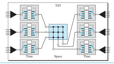
The last stage is a mirror image of the first stage. The middle stage is a space-division switch (crossbar) that connects the TSI groups to allow connectivity between all possible input and output pairs (e.g., to connect input 3 of the first group to output 7 of the second group).
