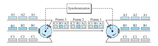
duration of a frame is therefore 1/100 s. The link is carrying 100 frames per second, and since each frame contains 32 bits, the bit rate is  $100 \times 32$ , or 3200 bps. This is actually 4 times the bit rate of each channel, which is  $100 \times 8 = 800$  bps.
