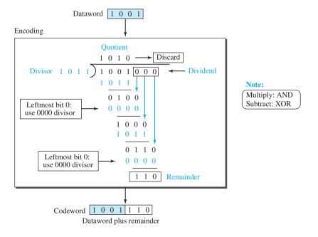
The process of modulo-2 binary division is the same as the familiar division process we use for decimal numbers. However, addition and subtraction in this case are the same; we use the XOR operation to do both.
