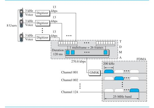
Twenty-six frames also share a multiframe (TDMA). We can calculate the bit rate of each channel as follows.
