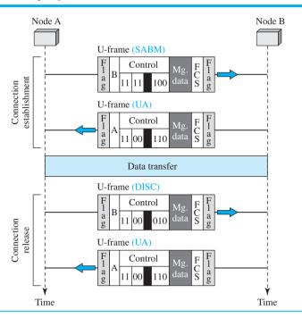
Figure 11.18 Example of connection and disconnection
