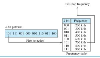
hops around from carrier to carrier. We assume the required bandwidth of the original signal is 100 kHz.
