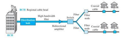
The **regional cable head (RCH)** normally serves up to 400,000 subscribers. The RCHs feed the **distribution hubs**, each of which serves up to 40,000 subscribers. The distribution hub plays an important role in the new infrastructure. Modulation and distribution of signals are done here; the signals are then fed to the fiber nodes through fiber-optic cables. The fiber node splits the analog signals so that the same signal is sent
