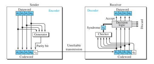
The calculation is done in **modular arithmetic** (see Appendix E). The encoder uses a generator that takes a copy of a 4-bit dataword ( $a_0$ ,  $a_1$ ,  $a_2$ , and  $a_3$ ) and generates a parity bit  $r_0$ . The dataword bits and the parity bit create the 5-bit codeword. The parity bit that is added makes the number of 1s in the codeword even. This is normally done by adding the 4 bits of the dataword (modulo-2); the result is the parity bit. In other words,
