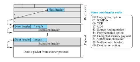
The payload in IPv6 means a combination of zero or more extension headers (options) followed by the data from other protocols (UDP, TCP, and so on). In IPv6, options, which are part of the header in IPv4, are designed as extension headers. The payload can have as many extension headers as required by the situation. Each extension header has two mandatory fields, next header and the length,
