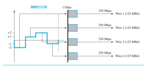
Figure 4.12 Multilevel: 4D-PAM5 scheme
