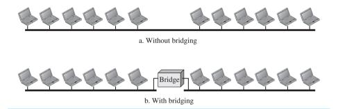
station in each segment), not 12 stations. In a network with a heavy load, each station theoretically is offered 10/7 Mbps instead of 10/12 Mbps.
