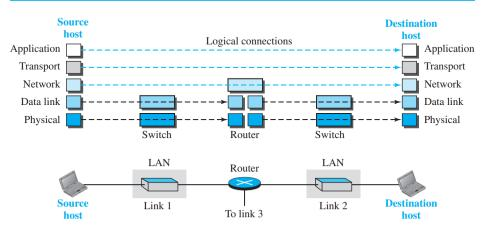
Using logical connections makes it easier for us to think about the duty of each layer. As the figure shows, the duty of the application, transport, and network layers is end-to-end. However, the duty of the data-link and physical layers is hop-to-hop, in which a hop is a host or router. In other words, the domain of duty of the top three layers is the internet, and the domain of duty of the two lower layers is the link.
