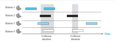
Figure 12.2 Frames in a pure ALOHA network
