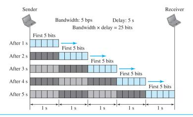
of bandwidth and delay; we need to fill up the full-duplex channel (two directions). The sender should send a burst of data of  $(2 \times \text{bandwidth} \times \text{delay})$  bits. The sender then waits for receiver acknowledgment for part of the burst before sending another burst. The amount  $2 \times \text{bandwidth} \times \text{delay}$  is the number of bits that can be in transition at any time.
