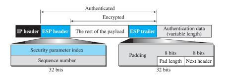
When an IP datagram carries an ESP header and trailer, the value of the protocol field in the IP header is 50. A field inside the ESP trailer (the next-header field) holds the original value of the protocol field (the type of payload being carried by the IP datagram, such as TCP or UDP). The ESP procedure follows these steps:
