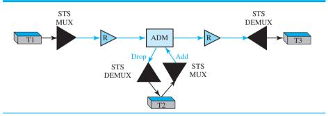
In Figure 14.32, T1 can send data to T2 and T3 simultaneously. T2, however, can send data only to T3. The figure shows a very simple configuration; in normal situations, we have more ADMs and more terminals.
