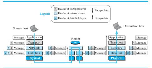
We have not shown the layers for the link-layer switches because no encapsulation/decapsulation occurs in this device. In Figure 2.8, we show the encapsulation in the source host, decapsulation in the destination host, and encapsulation and decapsulation in the router.
