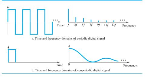
Note that both bandwidths are infinite, but the periodic signal has discrete frequencies while the nonperiodic signal has continuous frequencies.
