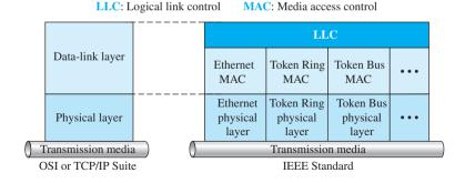
part of the framing duties are collected into one sublayer called the *logical link control* (LLC). Framing is handled in both the LLC sublayer and the MAC sublayer.
