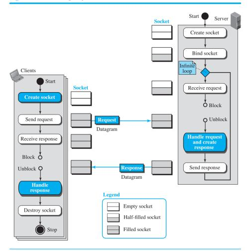
Figure 25.9 Flow diagram for iterative UDP communication
