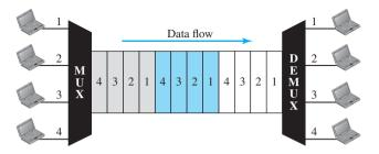
Note that in Figure 6.12 we are concerned with only multiplexing, not switching. This means that all the data in a message from source 1 always go to one specific destination, be it 1, 2, 3, or 4. The delivery is fixed and unvarying, unlike switching.
