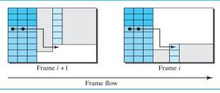
the beginning of the SPEs. Note that we need 2 bytes to define the position of a byte in a frame; a frame has 810 bytes, which cannot be defined using 1 byte.
