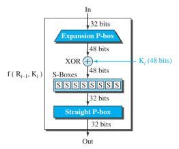
After the expansion permutation, DES uses the XOR operation on the expanded right section and the round key. The S-boxes do the real mixing. DES uses 8 S-boxes, each with a 6-bit input and a 4-bit output. The last operation in the DES function is a straight permutation with a 32-bit input and a 32-bit output.
