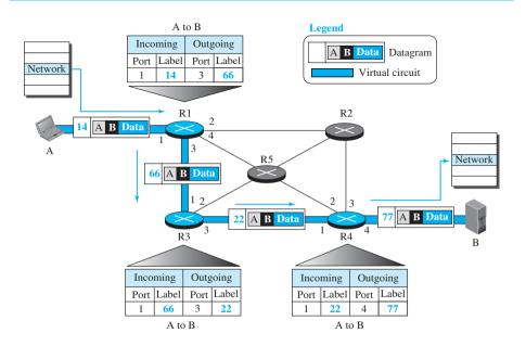
phase. Router R1 forwards the packet to router R3, but changes the label to 66. Router R3 forwards the packet to router R4, but changes the label to 22. Finally, router R4 delivers the packet to its final destination with the label 77. All the packets in the message follow the same sequence of labels, and the packets arrive in order at the destination
