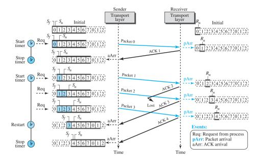
After initialization, there are some sender events. Request events are triggered by message chunks from the application layer; arrival events are triggered by ACKs received from the network layer. There is no time-out event here because all outstanding packets are acknowledged before the timer expires. Note that although ACK 2 is lost, ACK 3 is cumulative and serves as both ACK 2 and ACK 3. There are four events at the receiver site.
