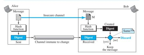
The two pairs (document/fingerprint) and (message/message digest) are similar, with some differences. The document and fingerprint are physically linked together. The message and message digest can be unlinked (or sent separately), and, most importantly, the message digest needs to be safe from change.
