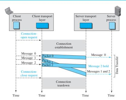
Figure 23.15 Connection-oriented service
