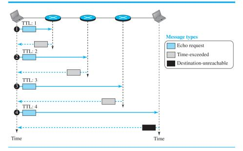
The *traceroute* program also sets a timer to find the round-trip time for each router and the destination. Most *traceroute* programs send three messages to each device, with the same TTL value, to be able to find a better estimate for the round-trip time. The following shows an example of a *traceroute* program, which uses three probes for each device and gets three RTTs.
