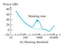
For example, we can save bits, without loss of quality, by omitting any sound with frequency of less than 100 Hz if its power is below 20 dB.
