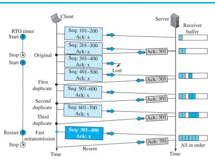
Figure 24.26 Fast retransmission
