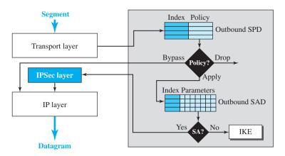
bypass (bypassing security header), and apply (applying the security according to the SAD; if no SAD, creating one).
