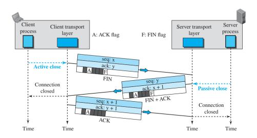
Figure 24.12 Connection termination using three-way handshaking
