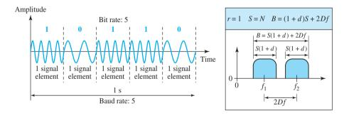
As Figure 5.6 shows, the middle of one bandwidth is  $f_1$  and the middle of the other is  $f_2$ . Both  $f_1$  and  $f_2$  are  $\Delta_f$  apart from the midpoint between the two bands. The difference between the two frequencies is  $2\Delta_f$ .
