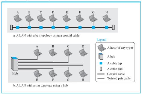
Figure 13.5 Implementation of standard Ethernet
