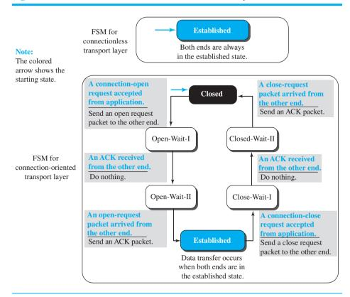
remote transport layer and moves to the *open-wait-I* state. When an acknowledgment is received from the other end, the local FSM moves to the *open-wait-II* state. When the machine is in this state, a unidirectional connection has been established, but if a bidirectional connection is needed, the machine needs to wait in this state until the other end also requests a connection. When the request is received, the machine sends an acknowledgment and moves to the *established* state.
