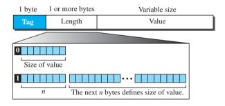
needed to define the length. The value field codes the value of the data according to the rules defined in BER.
