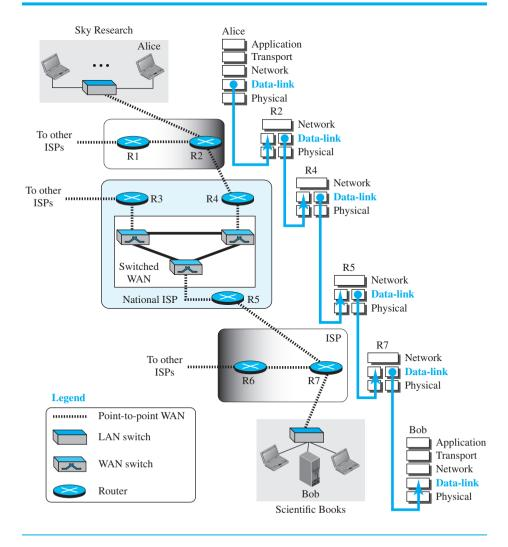
The data-link layer at Alice's computer communicates with the data-link layer at router R2. The data-link layer at router R2 communicates with the data-link layer at router R4,
