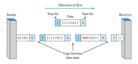
without the addition of control information. But it is cheap and effective, two advantages that make it an attractive choice for situations such as low-speed communication. For example, the connection of a keyboard to a computer is a natural application for asynchronous transmission. A user types only one character at a time, types extremely slowly in data processing terms, and leaves unpredictable gaps of time between characters
