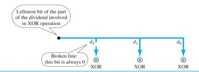
Note that if the leftmost bit of the part of the dividend to be used in this step is 1, the divisor bits  $(d_2d_1d_0)$  are 011; if the leftmost bit is 0, the divisor bits are 000. The design provides the right choice based on the leftmost bit.
