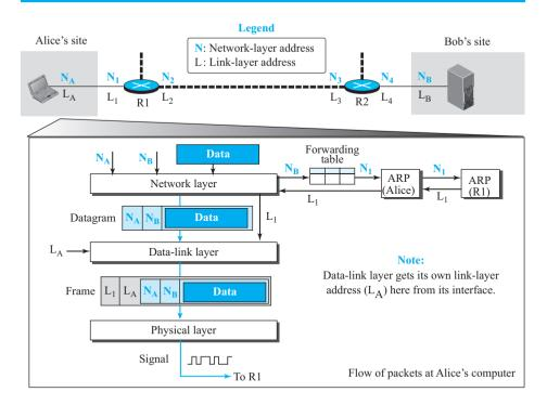
The network layer knows it's given  $N_A$ ,  $N_B$ , and the packet, but it needs to find the link-layer address of the next node. The network layer consults its routing table and tries to find which router is next (the default router in this case) for the destination  $N_B$ . As we will discuss in Chapter 18, the routing table gives  $N_1$ , but the network layer
