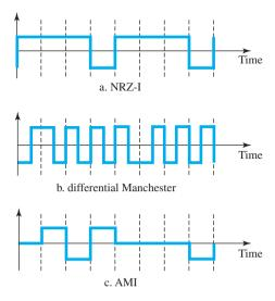
P4-10. An NRZ-I signal has a data rate of 100 Kbps. Using Figure 4.6, calculate the value of the normalized energy (P) for frequencies at 0 Hz, 50 KHz, and 100 KHz.
