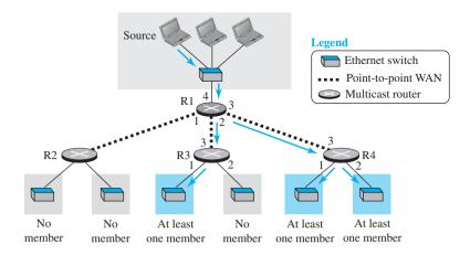
In multicasting, a multicast router may have to send out copies of the same data-gram through more than one interface. In Figure 21.2, router R1 needs to send out the data-gram through interfaces 2 and 3. Similarly, router R4 needs to send out the data-gram through both its interfaces. Router R3, however, knows that there is no member belonging to this group in the area reached by interface 2; it only sends out the data-gram through interface 1.
