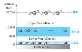
One reason for having different orbits is the existence of two Van Allen belts. A Van Allen belt is a layer that contains charged particles. A satellite orbiting in one of these two belts would be totally destroyed by the energetic charged particles. The MEO orbits are located between these two belts.
