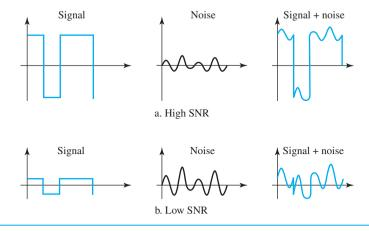
SNR is actually the ratio of what is wanted (signal) to what is not wanted (noise). A high SNR means the signal is less corrupted by noise; a low SNR means the signal is more corrupted by noise.
