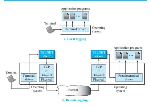
When a user logs into a local system, it is called *local logging*. As a user types at a terminal or at a workstation running a terminal emulator, the keystrokes are accepted by the terminal driver. The terminal driver passes the characters to the operating system. The operating system, in turn, interprets the combination of characters and invokes the desired application program or utility.
