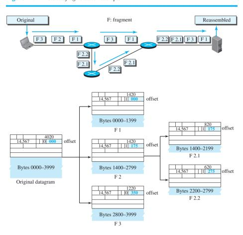
The figure also shows what happens if a fragment itself is fragmented. In this case the value of the offset field is always relative to the original datagram. For example, in the figure, the second fragment is itself fragmented later into two fragments of
