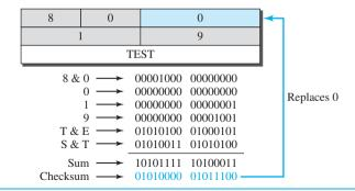
into 16-bit (2-byte) words. The words are added and the sum is complemented. Now the sender can put this value in the checksum field.
