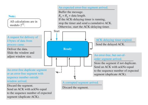
Again, there are some differences between this FSM and the one we discussed for an SR protocol. One difference is the ACK delaying in unidirectional communication. The other difference is the sending of duplicate ACKs to allow the sender to implement fast retransmission policy.
