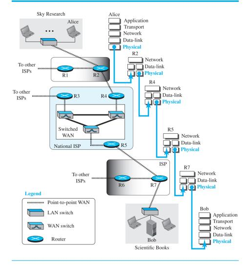
We can think of five different levels of communication between Alice, the computer on which our scientist is working, and Bob, the computer that provides online service. Communication at application, transport, network, or data-link is *logical*; communication at the physical layer is *physical*. For simplicity, we have shown only
