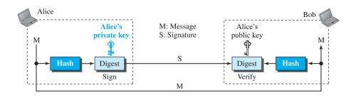
A digest is made out of the message at Alice's site. The digest then goes through the signing process using Alice's private key. Alice then sends the message and the signature to Bob.
