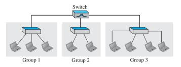
The first three engineers work together as the first group, the next two engineers work together as the second group, and the last four engineers work together as the third group. The LAN is configured to allow this arrangement.
