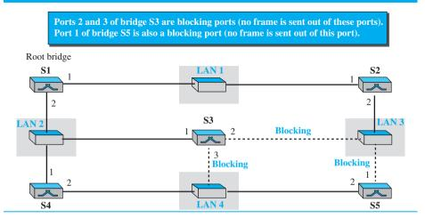
Note that there is only one path from any LAN to any other LAN in the spanning tree system. This means there is only one path from one LAN to any other LAN. No loops are created. You can prove to yourself that there is only one path from LAN 1 to LAN 2, LAN 3, or LAN 4. Similarly, there is only one path from LAN 2 to LAN 1, LAN 3, and LAN 4. The same is true for LAN 3 and LAN 4.
