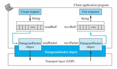
The design shows that we have a client socket object (of type DatagramSocket) created by the client program to provide a connection between the client and the transport layer (UDP). Since the application program delivers the data as a chunk, we need
