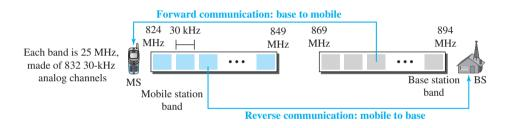
Each band is divided into 832 channels. However, two providers can share an area, which means 416 channels in each cell for each provider. Out of these 416, 21 channels are used for control, which leaves 395 channels. AMPS has a frequency reuse factor of 7; this means only one-seventh of these 395 traffic channels are actually available in a cell.
