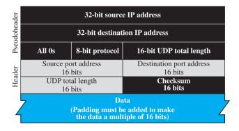
If the checksum does not include the pseudoheader, a user datagram may arrive safe and sound. However, if the IP header is corrupted, it may be delivered to the wrong host.
