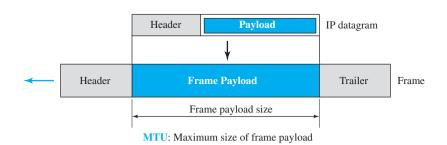
The value of the MTU differs from one physical network protocol to another. For example, the value for a LAN is normally 1500 bytes, but for a WAN it can be larger or smaller.
