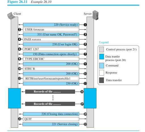
opened and closed repeatedly. We assume the file is transferred in six sections. After all records have been transferred, the server control process announces that the file transfer is done. Since the client control process has no file to retrieve, it issues the QUIT command, which causes the service connection to be closed.
