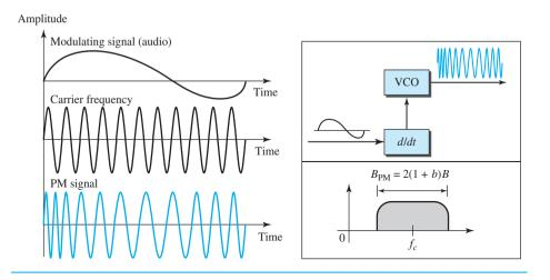
As Figure 5.20 shows, PM is normally implemented by using a voltage-controlled oscillator along with a derivative. The frequency of the oscillator changes according to the derivative of the input voltage, which is the amplitude of the modulating signal.
