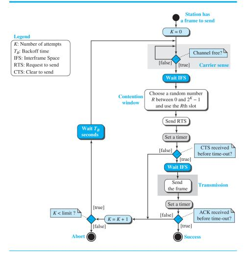
■ Interframe Space (IFS). First, collisions are avoided by deferring transmission even if the channel is found idle. When an idle channel is found, the station does not send immediately. It waits for a period of time called the interframe space or IFS. Even though the channel may appear idle when it is sensed, a distant station may have already started transmitting. The distant station's signal has not yet reached this
