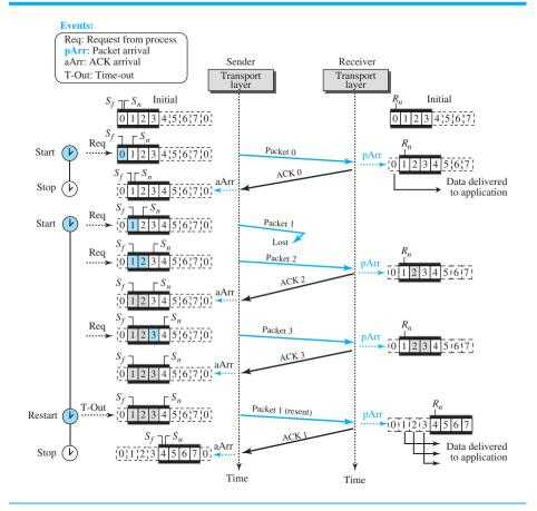
At the sender, packet 0 is transmitted and acknowledged. Packet 1 is lost. Packets 2 and 3 arrive out of order and are acknowledged. When the timer times out, packet 1 (the only unacknowledged packet) is resent and is acknowledged. The send window then slides.
