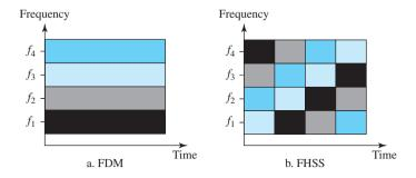
Figure 6.31 shows an example of four channels using FDM and four channels using FHSS. In FDM, each station uses 1/M of the bandwidth, but the allocation is fixed; in FHSS, each station uses 1/M of the bandwidth, but the allocation changes hop to hop.
