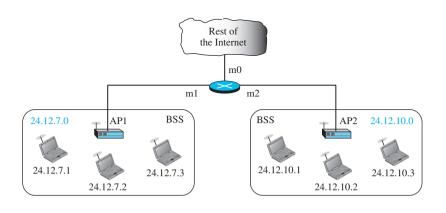
P15-11. In Figure 15.25 (previous problem), assume that the host with IP address 24.12.10.3 needs to send an IP datagram to the host with IP address 128.41.23.12 somewhere in the world (not shown in the figure). Explain the process and show how the values of address 1, address 2, address 3, and address 4 (see Figure 15.25) are determined in this case.
