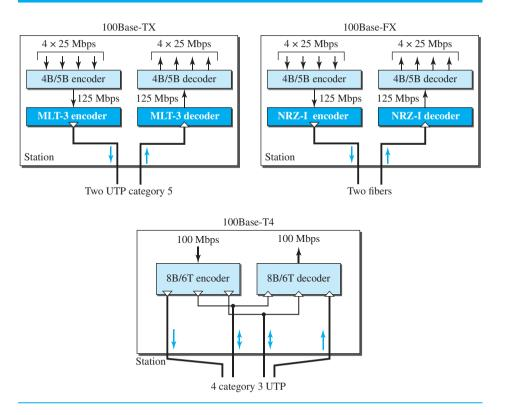
**100Base-TX** uses two pairs of twisted-pair cable (either category 5 UTP or STP). For this implementation, the MLT-3 scheme was selected since it has good bandwidth performance (see Chapter 4). However, since MLT-3 is not a self-synchronous line coding scheme, 4B/5B block coding is used to provide bit synchronization by preventing
