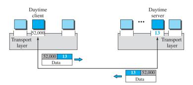
It should be clear by now that the IP addresses and port numbers play different roles in selecting the final destination of data. The destination IP address defines the host among the different hosts in the world. After the host has been selected, the port number defines one of the processes on this particular host (see Figure 23.4).
