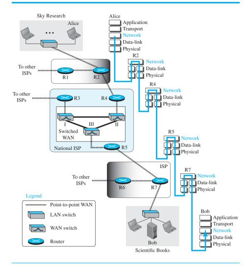
The figure shows that the Internet is made of many networks (or links) connected through the connecting devices. In other words, the Internet is an internetwork, a
