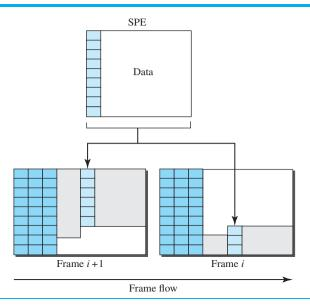
To find the beginning of each SPE in a frame, we need two pointers, H1 and H2, in the line overhead. Note that these pointers are located in the line overhead because the encapsulation occurs at a multiplexer. Figure 14.24 shows how these 2 bytes point to
