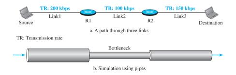
of 150 kbps, but there is not enough data to be sent. In other words, the average rate of the data flow in Link3 is also 100 kbps. We can conclude that the average data rate for this path is 100 kbps, the minimum of the three different data rates. The figure also shows that we can simulate the behavior of each link with pipes of different sizes; the average throughput is determined by the bottleneck, the pipe with the smallest diameter. In general, in a path with n links in series, we have
