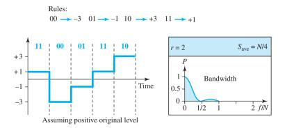
The average signal rate of 2B1Q is S = N/4. This means that using 2B1Q, we can send data 2 times faster than by using NRZ-L. However, 2B1Q uses four different signal levels, which means the receiver has to discern four different thresholds. The reduced bandwidth comes with a price. There are no redundant signal patterns in this scheme because  $2^2 = 4^1$ .
