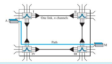
We have explicitly shown the multiplexing symbols to emphasize the division of the link into channels even though multiplexing can be implicitly included in the switch fabric.
