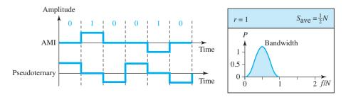
The bipolar scheme was developed as an alternative to NRZ. The bipolar scheme has the same signal rate as NRZ, but there is no DC component. The NRZ scheme has most of its energy concentrated near zero frequency, which makes it unsuitable for transmission over channels with poor performance around this frequency. The concentration of the energy in bipolar encoding is around frequency *N*/2. Figure 4.9 shows the typical energy concentration for a bipolar scheme.
