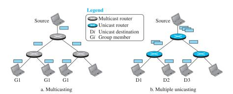
Figure 21.3 Multicasting versus multiple unicasting
