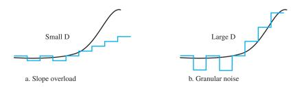
Since most functions have regions with both large and small slopes, selecting a large value or a small value for  $\Delta$  decreases one type of error but increases the other type. **Adaptive DM** (**ADM**) is used to solve the problem. In ADM, the value of  $\Delta$  changes from one step to the next and is calculated as shown below.
