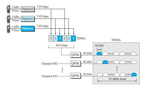
frame. Each frame lasts 40 ms (1/25) and is divided into six slots shared by three digital channels; each channel is allotted two slots.
