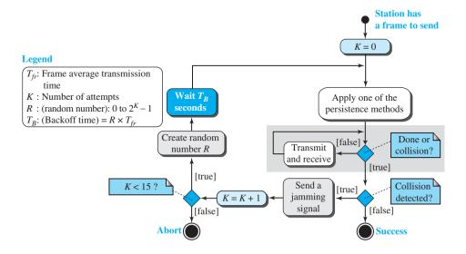
The first difference is the addition of the persistence process. We need to sense the channel before we start sending the frame by using one of the persistence processes we discussed previously (nonpersistent, 1-persistent, or *p*-persistent). The corresponding box can be replaced by one of the persistence processes shown in Figure 12.10.
