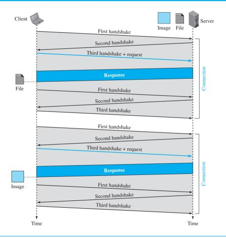
client and server are involved in two connection establishments and two connection terminations. If the transaction involves retrieving 10 or 20 objects, the round trip times spent for these handshakes add up to a big overhead. When we describe the client-server programming at the end of the chapter, we will show that for each connection the client and server need to allocate extra resources such as buffers and variables. This is another burden on both sites, but especially on the server site.
