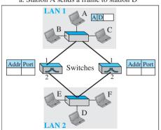
b. Both switches forward the frame
