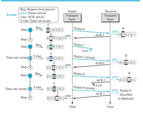
Figure 23.22 Flow diagram for Example 23.4
