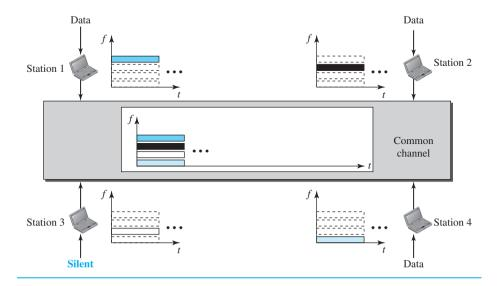
In FDMA, the available bandwidth of the common channel is divided into bands that are separated by guard bands.
