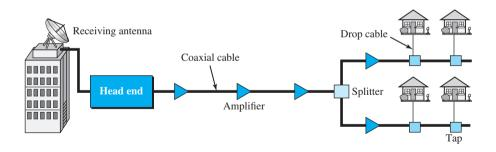
At the other end, splitters split the cable, and taps and drop cables made the connections to the subscriber premises.
