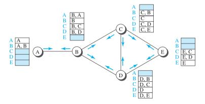
The policy is defined by selecting the *best* of multiple paths. Path-vector routing also imposes one more condition on this equation: If Path (v, y) includes x, that path is discarded to avoid a loop in the path. In other words, x does not want to visit itself when it selects a path to y.
