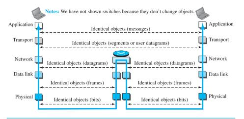
Note that, although the logical connection at the network layer is between the two hosts, we can only say that identical objects exist between two hops in this case because a router may fragment the packet at the network layer and send more packets than received (see fragmentation in Chapter 19). Note that the link between two hops does not change the object.
