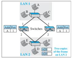
c. Both switches forward the frame
