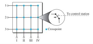
crossbar switch requires  $n \times m$  crosspoints. For example, to connect 1000 inputs to 1000 outputs requires a switch with 1,000,000 crosspoints. A crossbar switch [?] with this number of crosspoints is impractical. Such a switch is also inefficient because statistics show that, in practice, fewer than 25 percent of the crosspoints are in use at any given time. The rest are idle.
