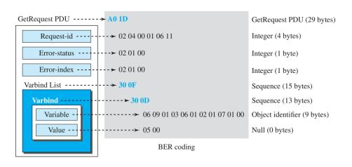
Figure 27.21 shows the actual message sent. We assume that the message header is made of 10 bytes. The actual message header may be different. We show the message using rows of 4 bytes. The bytes that are shown using dashes are the ones related to the message header.
