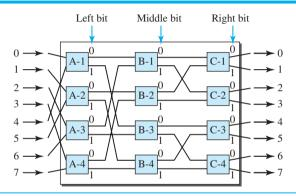
Figure 8.25 shows the operation. In part a, a packet has arrived at input port 1 and must go to output port 6 (110 in binary). The first microswitch (A-2) routes the packet
