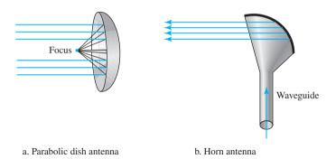
A **parabolic dish antenna** is based on the geometry of a parabola: Every line parallel to the line of symmetry (line of sight) reflects off the curve at angles such that all the lines intersect in a common point called the focus. The parabolic dish works as a funnel, catching a wide range of waves and directing them to a common point. In this way, more of the signal is recovered than would be possible with a single-point receiver.
