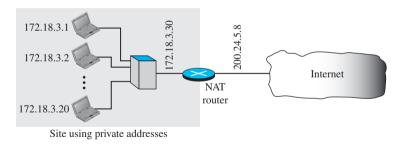
As the figure shows, the private network uses private addresses. The router that connects the network to the global address uses one private address and one global address. The private network is invisible to the rest of the Internet; the rest of the Internet sees only the NAT router with the address 200.24.5.8.
