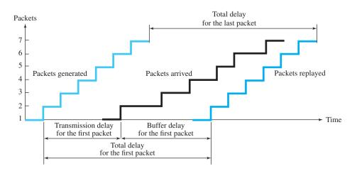
As the figure shows, if the playback time for the first packet is selected properly, then the total delay for all packets should be the same. The packets that have longer transmission delay should have shorter waiting in the buffer and vice versa.
