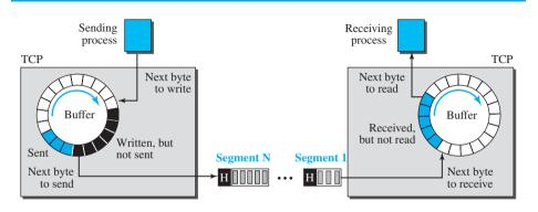
Note that segments are not necessarily all the same size. In the figure, for simplicity, we show one segment carrying 3 bytes and the other carrying 5 bytes. In reality, segments carry hundreds, if not thousands, of bytes.
