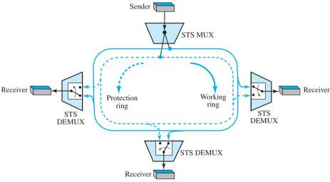
Although we have chosen one sender and three receivers in the figure, there can be many other configurations. The sender uses a two-way connection to send data to both rings simultaneously; the receiver uses selecting switches to select the ring with better signal quality. We have used one STS multiplexer and three STS demultiplexers to emphasize that nodes operate on the path layer.
