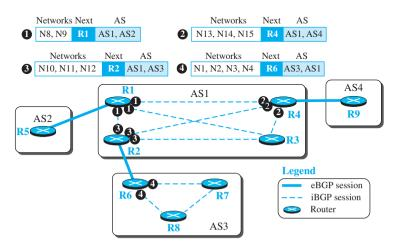
Note that we have not shown the physical networks inside ASs because a session is made on an overlay network (TCP connection), possibly spanning more than one physical network as determined by the route dictated by intradomain routing protocol. Also note that in this stage only four messages are exchanged. The first message (numbered 1) is sent by R1 announcing that networks N8 and N9 are reachable through the
