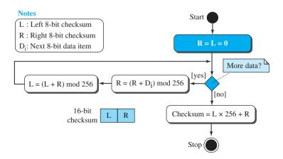
Figure 10.19 Algorithm to calculate an Adler checksum
