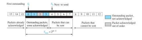
window that are shaded define packets that have arrived out of order and are waiting for the earlier transmitted packet to arrive before delivery to the application layer.
