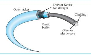
made of either PVC or Teflon. Inside the jacket are Kevlar strands to strengthen the cable. Kevlar is a strong material used in the fabrication of bulletproof vests. Below the Kevlar is another plastic coating to cushion the fiber. The fiber is at the center of the cable, and it consists of cladding and core.
