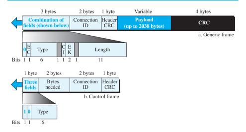
The first bit in a frame is the frame identifier. If it is 0, the frame is a generic frame; if
