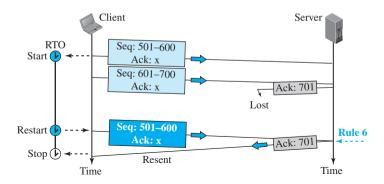
If the next acknowledgment is delayed for a long time or there is no next acknowledgment (the lost acknowledgment is the last one sent), the correction is triggered by the RTO timer. A duplicate segment is the result. When the receiver receives a duplicate segment, it discards it and resends the last ACK immediately to inform the sender that the segment or segments have been received.
