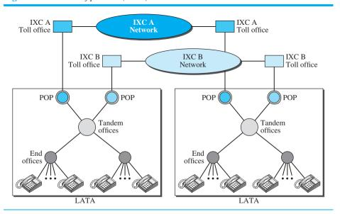
A subscriber who needs to make a connection with another subscriber is connected first to an end switch and then, either directly or through a tandem switch, to a POP. The call now goes from the POP of an IXC (the one the subscriber has chosen) in the source LATA to the POP of the same IXC in the destination LATA. The call is passed through the toll office of the IXC and is carried through the network provided by the IXC.
