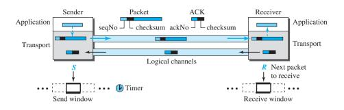
The Stop-and-Wait protocol is a connection-oriented protocol that provides flow and error control.
