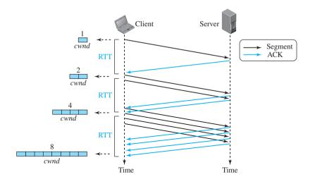
the size of the congestion window in this algorithm is a function of the number of ACKs arrived and can be determined as follows.
