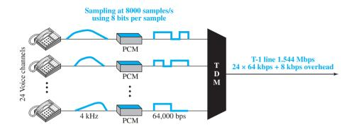
**The T-1 Frame** As noted above, DS-1 requires 8 kbps of overhead. To understand how this overhead is calculated, we must examine the format of a 24-voice-channel frame.
