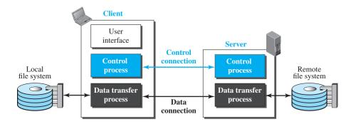
basic model of FTP. The client has three components: the user interface, the client control process, and the client data transfer process. The server has two components: the server control process and the server data transfer process. The control connection is made between the control processes. The data connection is made between the data transfer processes.
