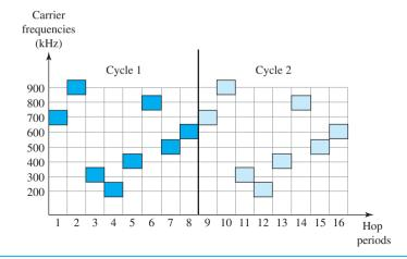
other words, M different stations can use the same  $B_{\rm ss}$  if an appropriate modulation technique such as multiple FSK (MFSK) is used. FHSS is similar to FDM, as shown in Figure 6.31.
