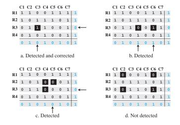
Show how the following errors can be detected:
