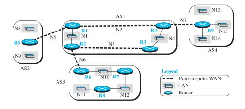
Each autonomous system in this figure uses one of the two common intradomain protocols, RIP or OSPF. Each router in each AS knows how to reach a network that is in its own AS, but it does not know how to reach a network in another AS.
