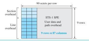
*payload envelope* (*SPE*). It contains user data and **path overhead** (**POH**) needed at the user data level. We will discuss the format of the SPE shortly.
