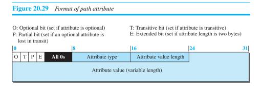
The first byte in each attribute defines the four attribute flags (as shown in the figure). The next byte defines the type of attributes assigned by ICANN (only seven types have been assigned, as explained next). The attribute value length defines the length of the attribute value field (not the length of the whole attributes section). The following gives a brief description of each attribute.
