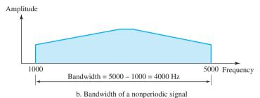
**Figure 3.14** The bandwidth for Example 3.10
