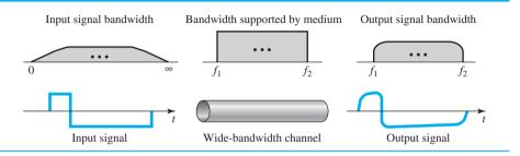
Although the output signal is not an exact replica of the original signal, the data can still be deduced from the received signal. Note that although some of the frequencies are blocked by the medium, they are not critical.
