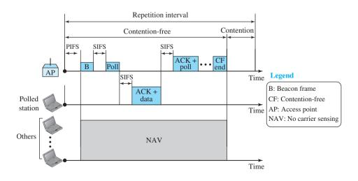
uses piggybacking). At the end of the contention-free period, the PC sends a CF end (contention-free end) frame to allow the contention-based stations to use the medium.
