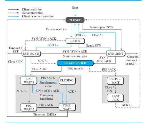
The state marked *ESTABLISHED* in the FSM is in fact two different sets of states that the client and server undergo to transfer data.
