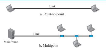
In a multipoint environment, the capacity of the channel is shared, either spatially or temporally. If several devices can use the link simultaneously, it is a *spatially shared* connection. If users must take turns, it is a *timeshared* connection.
