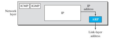
Anytime a host or a router needs to find the link-layer address of another host or router in its network, it sends an ARP request packet. The packet includes the link-layer and IP addresses of the sender and the IP address of the receiver. Because the sender does not know the link-layer address of the receiver, the query is broadcast over the link using the link-layer broadcast address, which we discuss for each protocol later (see Figure 9.7).
