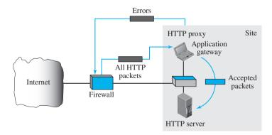
A proxy firewall filters at the application layer.
