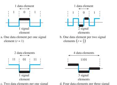
Finally, in part d, a group of 4 bits is being carried by a group of three signal elements (r = 4/3). For every line coding scheme we discuss, we will give the value of r.
