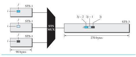
Note that a byte in an STS-1 frame keeps its row position, but it is moved into a different column. The reason is that while all signal frames have the same number of rows (9), the number of columns changes. The number of columns in an STS-*n* signal frame is *n* times the number of columns in an STS-1 frame. One STS-*n* row, therefore, can accommodate all *n* rows in the STS-1 frames.
