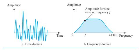
In a time-domain representation of this composite signal, there are an infinite number of simple sine frequencies. Although the number of frequencies in a human voice is infinite, the range is limited. A normal human being can create a continuous range of frequencies between 0 and 4 kHz.
