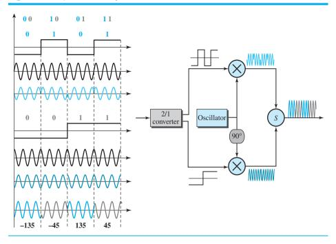
The two composite signals created by each multiplier are sine waves with the same frequency, but different phases. When they are added, the result is another sine wave, with one of four possible phases:  $45^{\circ}$ ,  $-45^{\circ}$ ,  $135^{\circ}$ , and  $-135^{\circ}$ . There are four kinds of signal elements in the output signal (L=4), so we can send 2 bits per signal element (r=2).
