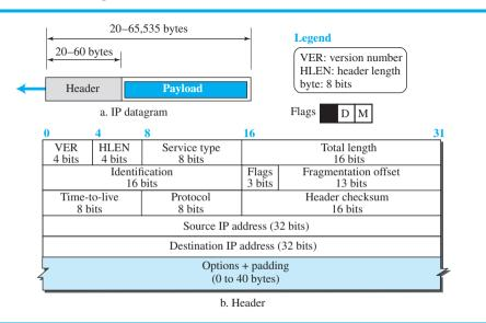
Discussing the meaning and rationale for the existence of each field is essential to understanding the operation of IPv4; a brief description of each field is in order.
