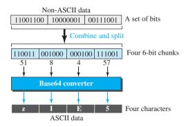
Each 6-bit section is then converted into an ASCII character according to Table 26.10.
