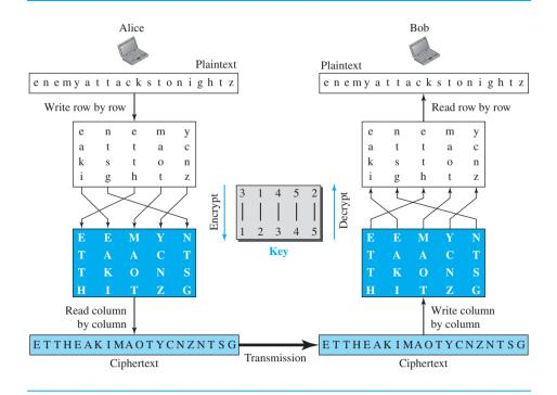
The first table is created by Alice writing the plaintext row by row. The columns are permuted using a key. The ciphertext is created by reading the second table column by column. Bob does the same three steps in the reverse order. He writes the ciphertext column by column into the first table, permutes the columns, and then reads the second table row by row. Note that the same key is used for encryption and decryption, but the algorithm uses the key in reverse order.
