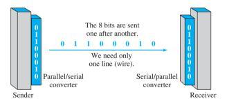
The advantage of serial over parallel transmission is that with only one communication channel, serial transmission reduces the cost of transmission over parallel by roughly a factor of n.
