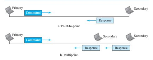
Figure 11.15 Asynchronous balanced mode
