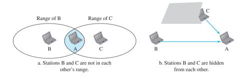
outside the transmission range of B; likewise, station B is outside the transmission range of C. Station A, however, is in the area covered by both B and C; it can hear any signal transmitted by B or C. The figure also shows that the hidden station problem may also occur due to an obstacle.
