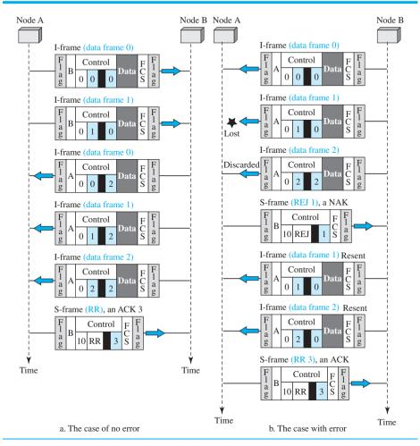
Figure 11.19 Example of piggybacking with and without error
