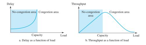
become full and the routers have to discard some packets. Discarding packets does not reduce the number of packets in the network because the sources retransmit the packets, using time-out mechanisms, when the packets do not reach the destinations.
