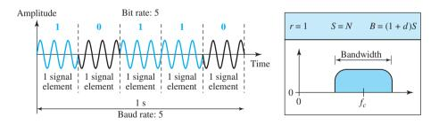
signal; in PSK, it is the phase. Noise can change the amplitude easier than it can change the phase. In other words, PSK is less susceptible to noise than ASK. PSK is superior to FSK because we do not need two carrier signals. However, PSK needs more sophisticated hardware to be able to distinguish between phases.
