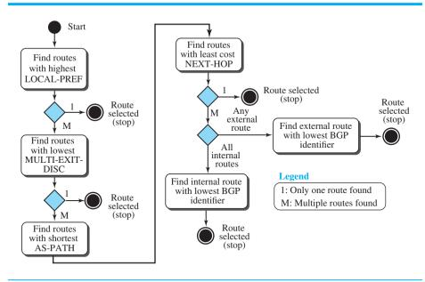
Figure 20.30 Flow diagram for route selection
