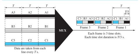
In synchronous TDM, a round of data units from each input connection is collected into a frame (we will see the reason for this shortly). If we have n connections, a frame is divided into n time slots and one slot is allocated for each unit, one for each input line. If the duration of the input unit is T, the duration of each slot is T/n and the duration of each frame is T (unless a frame carries some other information, as we will see shortly).
