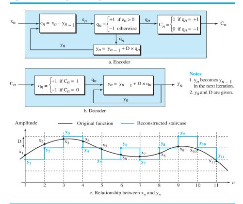
function. Quantizing  $x_n - y_{n-1}$  is self-correcting for slow-growing or slow-falling x. Figure 28.10 compares the staircase reconstruction of quantizing  $x_n - x_{n-1}$  versus  $x_n - y_{n-1}$  for a slow-growing function. (For a slow-falling function, the idea is similar.)
