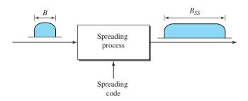
After the signal is created by the source, the spreading process uses a spreading code and spreads the bandwidth. The figure shows the original bandwidth B and the spread bandwidth  $B_{SS}$ . The spreading code is a series of numbers that look random, but are actually a pattern.
