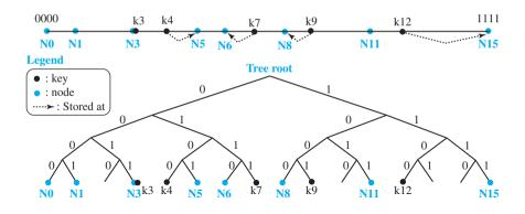
row. The idea is the same as that used by Pastry, but the length of the common prefix is based on the number of bits instead of the number of digits in base  $2^b$ . Table 29.8 shows the routing table.
