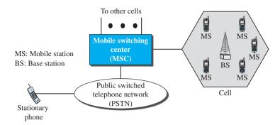
Cell size is not fixed and can be increased or decreased depending on the population of the area. The typical radius of a cell is 1 to 12 mi. High-density areas require more, geographically smaller cells to meet traffic demands than do low-density areas. Once determined, cell size is optimized to prevent the interference of adjacent cell signals. The transmission power of each cell is kept low to prevent its signal from interfering with those of other cells.
