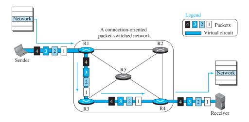
Each packet is forwarded based on the label in the packet. To follow the idea of connection-oriented design to be used in the Internet, we assume that the packet has a label when it reaches the router. Figure 18.6 shows the idea. In this case, the forwarding decision is based on the value of the label, or *virtual circuit identifier*, as it is sometimes called.
