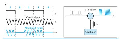
If digital data are presented as a unipolar NRZ (see Chapter 4) digital signal with a high voltage of 1 V and a low voltage of 0 V, the implementation can achieved by multiplying the NRZ digital signal by the carrier signal coming from an oscillator. When the amplitude of the NRZ signal is 1, the amplitude of the carrier frequency is held; when the amplitude of the NRZ signal is 0, the amplitude of the carrier frequency is zero.
