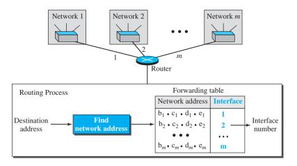
found, the router consults its forwarding table to find the corresponding interface from which the packet should be sent out. The network address is actually the identifier of the network; each network is identified by its network address.
