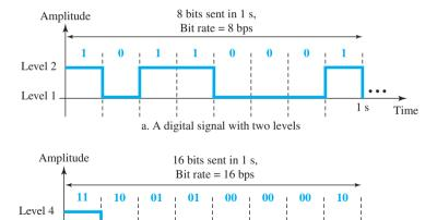
b. A digital signal with four levels
