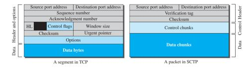
segment in TCP and a packet in SCTP. We will discuss the format of the SCTP packet in the next section.
