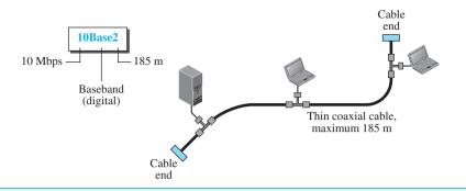
Note that the collision here occurs in the thin coaxial cable. This implementation is more cost effective than 10Base5 because thin coaxial cable is less expensive than thick coaxial and the tee connections are much cheaper than taps. Installation is simpler because the thin coaxial cable is very flexible. However, the length of each segment cannot exceed 185 m (close to 200 m) due to the high level of attenuation in thin coaxial cable.
