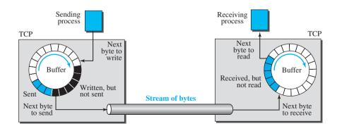
bytes that can be read by the receiving process. When a byte is read by the receiving process, the chamber is recycled and added to the pool of empty chambers.
