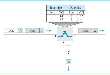
Figure 8.12 shows a frame arriving at port 1 with a VCI of 14. When the frame arrives, the switch looks in its table to find port 1 and a VCI of 14. When it is found, the switch knows to change the VCI to 22 and send out the frame from port 3.
