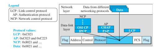
All LCP packets are carried in the payload field of the PPP frame with the protocol field set to C021 in hexadecimal (see Figure 11.23).
