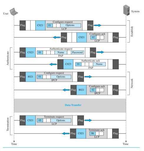
The first two frames show link establishment. We have chosen two options (not shown in the figure): using PAP for authentication and suppressing the address control fields. Frames 3 and 4 are for authentication. Frames 5 and 6 establish the network layer connection using IPCP.
