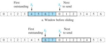
b. Window after sliding (an ACK with ackNo = 6 has arrived)
