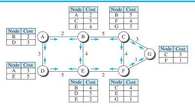
We can compare the link-state routing algorithm with the distance-vector routing algorithm. In the distance-vector routing algorithm, each router tells its neighbors what it knows about the whole internet; in the link-state routing algorithm, each router tells the whole internet what it knows about its neighbors.
