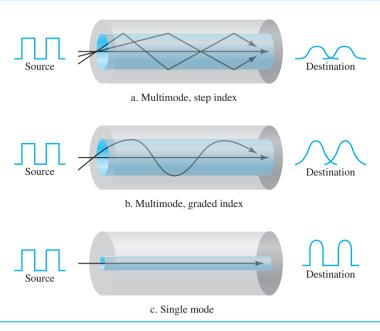
In **multimode step-index fiber**, the density of the core remains constant from the center to the edges. A beam of light moves through this constant density in a straight line until it reaches the interface of the core and the cladding. At the interface, there is an abrupt change due to a lower density; this alters the angle of the beam's motion. The term *step-index* refers to the suddenness of this change, which contributes to the distortion of the signal as it passes through the fiber.
