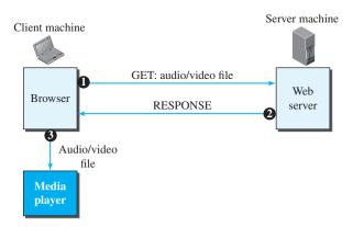
This approach is very simple and does not involve *streaming*. However, it has a drawback. An audio/video file is usually large even after compression. An audio file may contain tens of megabits, and a video file may contain hundreds of megabits. In this approach, the file needs to download completely before it can be played. Using contemporary data rates, the user needs some seconds or tens of seconds before the file can be played.
