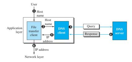
server name, such as *afilesource.com*. However, the TCP/IP suite needs the IP address of the file transfer server to make the connection. The following six steps map the host name to an IP address:
