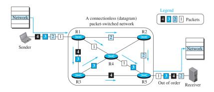
Each packet is routed based on the information contained in its header: source and destination addresses. The destination address defines where it should go; the source address defines where it comes from. The router in this case routes the packet based only on the destination address. The source address may be used to send an error message to the source if the packet is discarded. Figure 18.4 shows the forwarding process in a router in this case. We have used symbolic addresses such as A and B.
