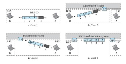
AP and going to a station. The addresses are as shown in Figure 15.11. Note that address 3 contains the original sender of the frame (in another BSS).
