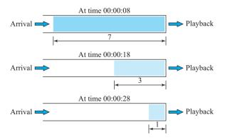
smoothly, as though there were no delay. Figure 28.32 shows the idea using the time line for seven packets. Note that we need to select the buffer delay for the first packet in the buffer in a such a way that the right two saw-tooth curves do not overlap.
