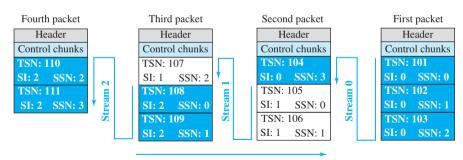
Flow of packets from sender to receiver
