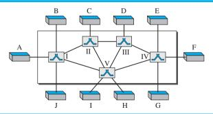
The **end systems** (communicating devices) are labeled A, B, C, D, and so on, and the switches are labeled I, II, III, IV, and V. Each switch is connected to multiple links.
