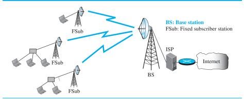
The fixed service can be compared with the service provided by the telephone and the network companies using wired connections. WiMAX also uses a MIMO antenna system, which can provide simultaneous transmitting and receiving.
