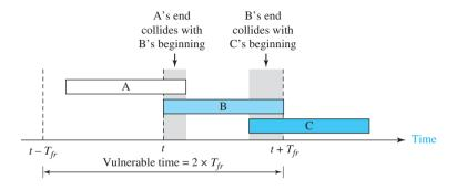
Station B starts to send a frame at time t. Now imagine station A has started to send its frame after  $t - T_{fr}$ . This leads to a collision between the frames from station B and
