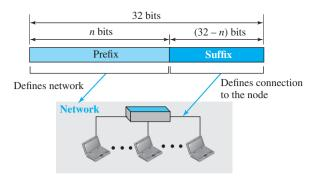
A prefix can be fixed length or variable length. The network identifier in the IPv4 was first designed as a fixed-length prefix. This scheme, which is now obsolete, is referred to as classful addressing. The new scheme, which is referred to as classless addressing, uses a variable-length network prefix. First, we briefly discuss classful addressing; then we concentrate on classless addressing.
