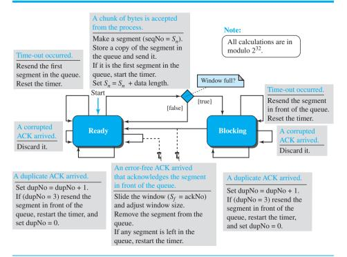
FSM is rudimentary; it does not include issues such as silly window syndrome (Nagle's algorithm) or window shutdown. It defines a unidirectional communication, ignoring all issues that affect bidirectional communication.
