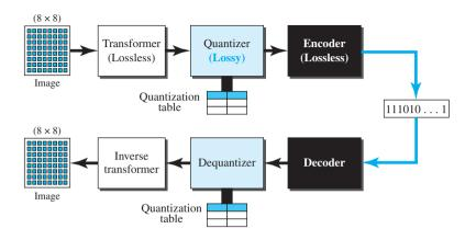
The purpose of dividing the picture into blocks is to decrease the number of calculations, because, as we showed in two-dimensional DCT, the number of mathematical operations for each picture is the square of the number of units.
