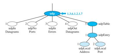
However, these object identifiers define the variable, not the instance (contents). To show the instance, or the contents, of each variable, we must add an instance suffix. The instance suffix for a simple variable is simply a zero. In other words, to show an instance of the above variables, we use the following:
