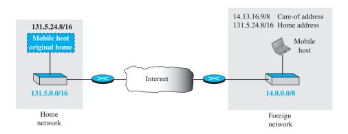
Mobile IP has two addresses for a mobile host: one home address and one care-of address. The home address is permanent; the care-of address changes as the mobile host moves from one network to another.
