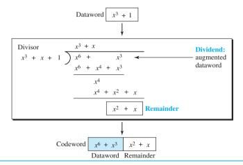
It can be seen that the polynomial representation can easily simplify the operation of division in this case, because the two steps involving all-0s divisors are not needed here. (Of course, one could argue that the all-0s divisor step can also be eliminated in binary division.) In a polynomial representation, the divisor is normally referred to as the *generator polynomial* t(x).
