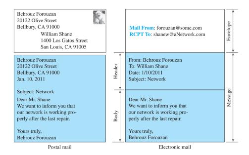
contains the *header* and the *body*. The header of the message defines the sender, the receiver, the subject of the message, and some other information. The body of the message contains the actual information to be read by the recipient.
