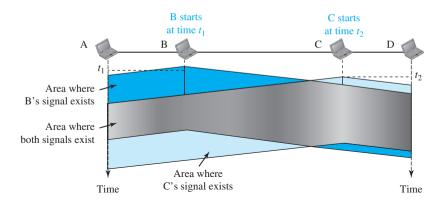
At time  $t_1$ , station B senses the medium and finds it idle, so it sends a frame. At time  $t_2$  ( $t_2 > t_1$ ), station C senses the medium and finds it idle because, at this time, the first bits from station B have not reached station C. Station C also sends a frame. The two signals collide and both frames are destroyed.
