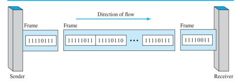
The advantage of synchronous transmission is speed. With no extra bits or gaps to introduce at the sending end and remove at the receiving end, and, by extension, with fewer bits to move across the link, synchronous transmission is faster than asynchronous transmission. For this reason, it is more useful for high-speed applications such as the transmission of data from one computer to another. Byte synchronization is accomplished in the data-link layer.
