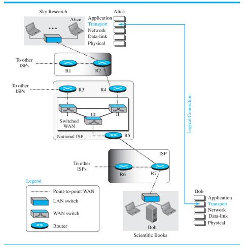
The figure shows the same scenario we used in Chapter 3 for the physical layer (Figure 3.1). Alice's host in the Sky Research company creates a logical connection with Bob's host in the Scientific Books company at the transport layer. The two compa-
