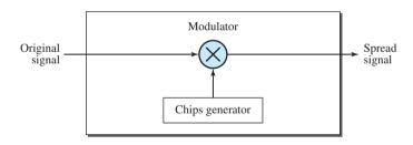
As an example, let us consider the sequence used in a wireless LAN, the famous **Barker sequence**, where n is 11. We assume that the original signal and the chips in the chip generator use polar NRZ encoding. Figure 6.33 shows the chips and the result of multiplying the original data by the chips to get the spread signal.
