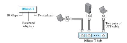
Note that two pairs of twisted cable create two paths (one for sending and one for receiving) between the station and the hub. Any collision here happens in the hub. Compared to 10Base5 or 10Base2, we can see that the hub actually replaces the coaxial cable as far as a collision is concerned. The maximum length of the twisted cable here is defined as 100 m, to minimize the effect of attenuation in the twisted cable.
