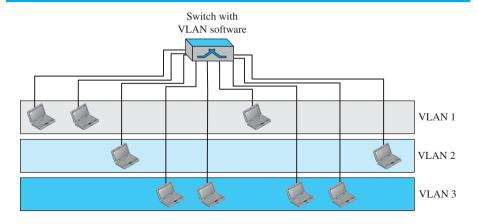
VLAN 2, it receives broadcast messages sent to VLAN 2, but no longer receives broadcast messages sent to VLAN 1.
