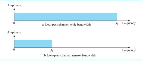
Let us study two cases of a baseband communication: a low-pass channel with a wide bandwidth and one with a limited bandwidth.
