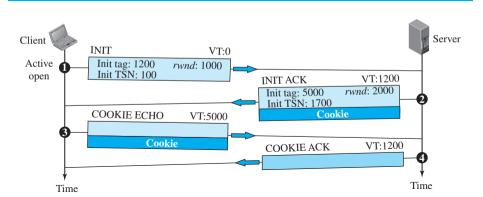
Figure 24.45 Four-way handshaking
