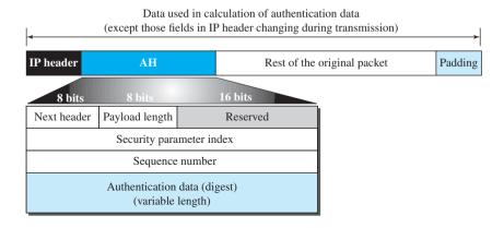
**5.** The IP header is added after changing the value of the protocol field to 51.
