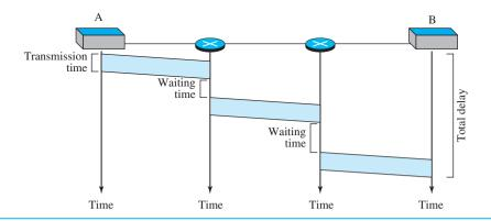
The packet travels through two switches. There are three transmission times (3T), three propagation delays (slopes  $3\tau$  of the lines), and two waiting times  $(w_1 + w_2)$ . We ignore the processing time in each switch. The total delay is
